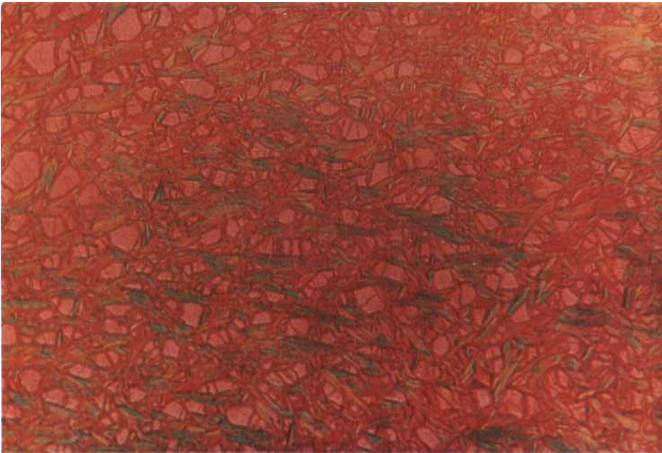
Figure 9. The 'platelet' texture of the S_A^* phase for the 25.3 mol% mixture.
